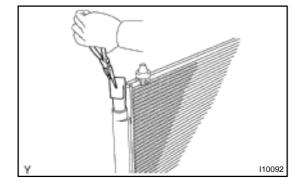
(c) Using pliers, remove the dryer.
