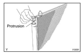
(e) Insert the filter into the modulator.
